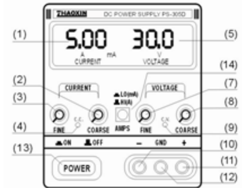
Picture 3 PS Series 3 digit LED display
