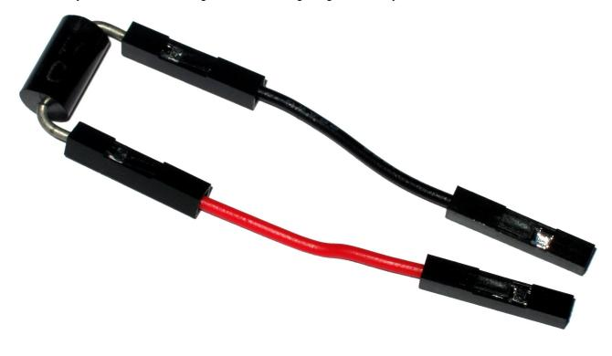
The leads on a 3A diode are slightly thicker that a male header pin. Bend the leads close to the body of the diode as shown and fit two small female-to-female jumper wires. They will be a tight fit but this is good as it ensures a good electrical connection. Fit a red wire to the anode and a black wire to the cathode.
