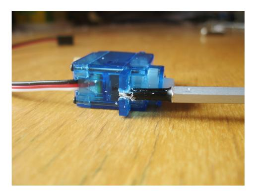
Once you have the 3mm screw in all the way, continue turning the screw a few times so that the screw thread can drill out the hole a bit more.
