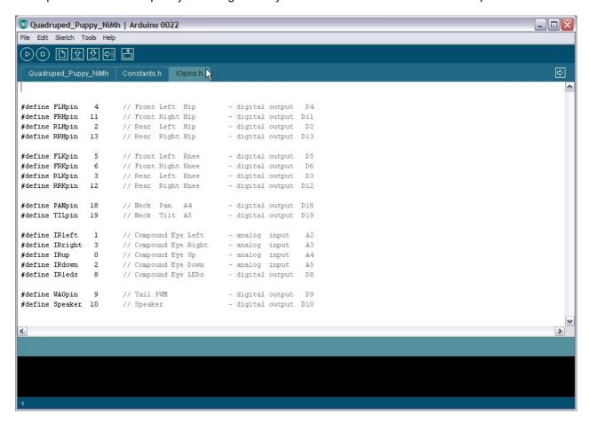
Go to the tools menu and select your board type. The Magician controller comes with either the ATmega8A or the ATmega328. If you have the ATmega8A then select "Arduino NG or older /w ATmega8". If your controller has the ATmega328 then select "Arduino Duemilanova or Nano /w ATmega328.
