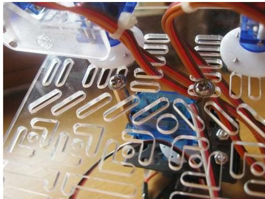
Use two 3 x 10mm pan head machine screws to mount the head. Notice the holes used in the first photo. The servo is mounted slightly to one side so that the pan servo's output shaft is centered rather than the servo body. The pan servo is mounted a reasonable distance back to improve the balance of the robot and to help protect the pan servo if the robot runs into a wall.
