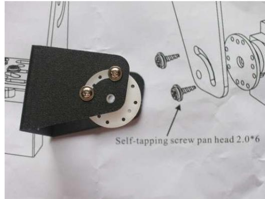
Use two 2 x 6mm pan head screws to attach a round servo horn to the tilt bracket. Use holes that will allow the center hole of the servo horn to align with the bracket as shown without allowing too much play if the screws come loose.
